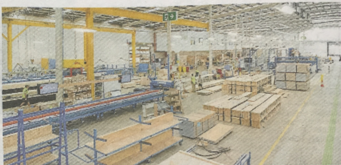
Strongbuild is producing prefabricated timber panels at its Baulkham Hills factory in Sydney.
